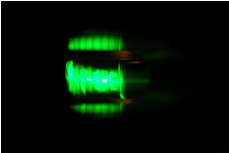
The beam phase-slipping about 3 in. out as it also hits a resonance
