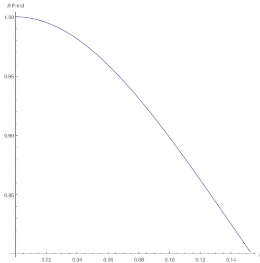
B field for simulation as function of Rutgers 12” radius
