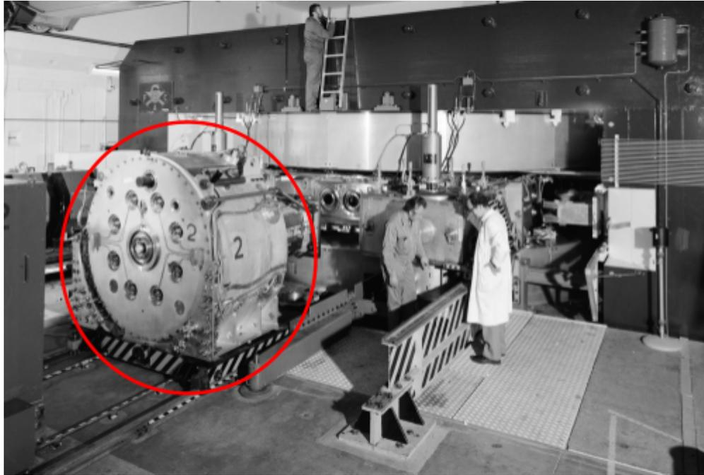
The rotary capacitor of the CERN 600 MeV Synchrocyclotron, circled [8]
