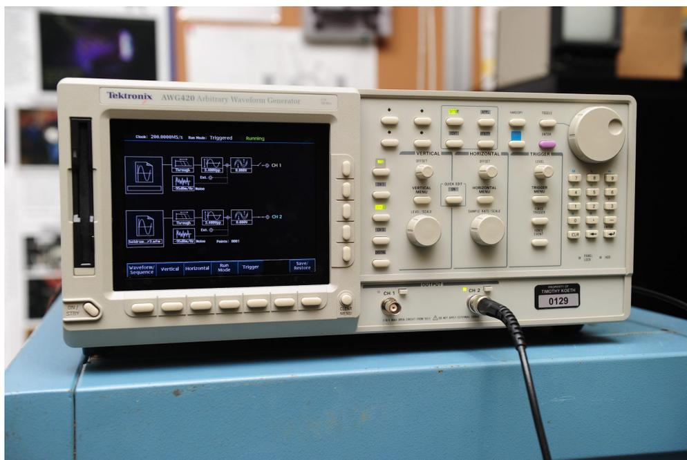
Tektronix AWG420, running the frequency-ramped function at a 1kHz rate
